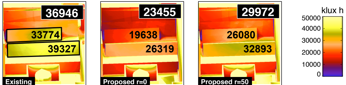
Figure 2. Illumination maps for the ASL skylights. Annotation shows total annual illuminance across the skylights. Inset value shows area-weighted mean. The view is a "close-up" of the skylights identified in blue in Figure 1.
